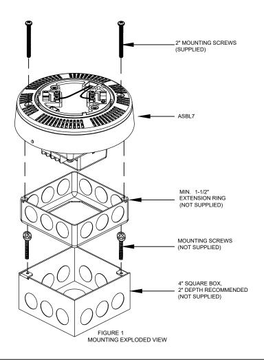
For Installations which extend beyond the mounting surface, or do not have sufficient mounting box depth, an optional trim ring is available. Insert the ASBL7 into the trim ring prior to mounting to the electrical box.
